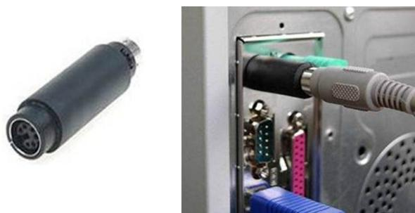
New storing device fits at the end of the keyboard cable connecting to the PC specialized to save all typed keys in it.
