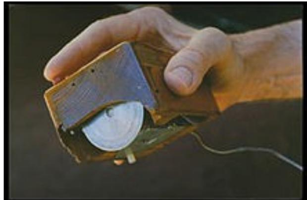
The first computer mouse, held by inventor Douglas Engelbart, showing the wheels that make contact with the working surface
