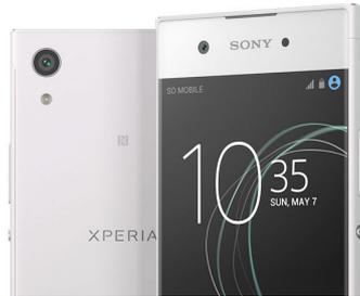
camera. It runs a MediaTek Helio P20 octacore processor (4 x 2.3GHz and 4 x 1.6GHz) supported by 3GB of RAM. There's 32GB of built in storage and you can add a microSD memory card of up to 256GB.
