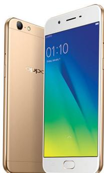
The phone runs a Qualcomm MSM8940 Octa-core processor (with 3GB of RAM). That processor is, according to the Internet, otherwise known as a Snapdragon 435 processor. According to the Qualcomm spec sheet, it supports Cat 7 data downloads up to 300 megabits per second, and Cat 13 uploads to 150Mbps.
